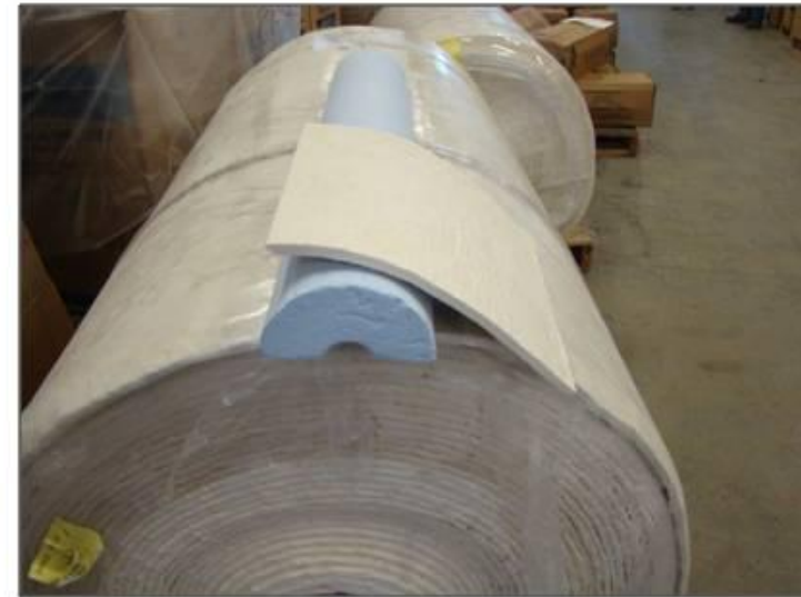
Pyrogel XT equivalent thickness to preformed insulation.
